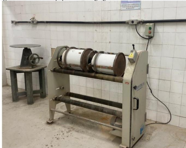
Figure 5 : Ball mill equipment belonging to the LEMAC/UFPA laboratory
