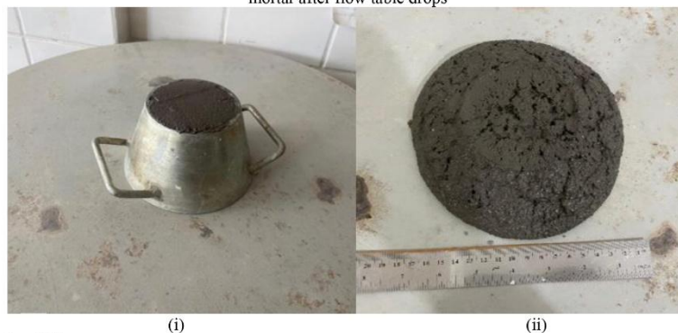
Figure10: Consistency index test on the processed EAF slag sample (i) mortar molded in the truncated cone (ii) mortar after flow table drops
