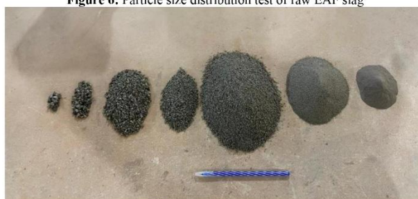
Figure 6: Particle size distribution test of raw EAF slag
